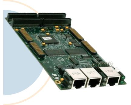
The EP 8280 computing engine takes advantage of the high performance networking capabilities of the Motorola Power PC 8280, Power PC 8270, Power PC 8266, Power PC 8265 or Power PC 8250 processor.
