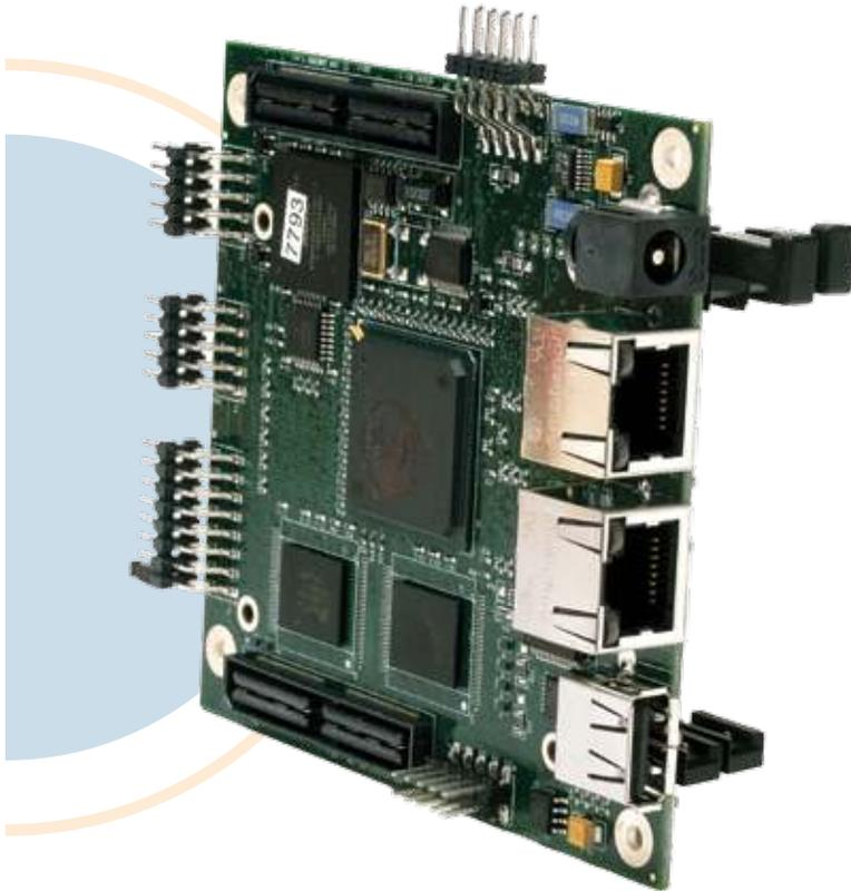
The EP885C uses the newest generation of Freescale's PowerQUICC I family, MPC885 and MPC880, to create a full featured PC/104 mechanical CPU module.
