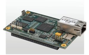
Access to the PRU and ADC features of the 437x are available. Uboot and Linux software are also available for the EP4376.
